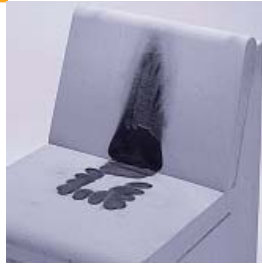
As shown in the photo, the foam August uses for CA133 does not support combustion.
